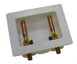
Boxes are supplied with water hammer arrestors and quarter turn valves. Boxes include necessary mounting brackets and faceplate. Plastic boxes are molded from high impact polystyrene and include a 2" female outlet for drain connection. (Note: Box dimensions may vary slightly from drawings).
